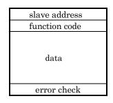
2) Communication command format (MODBUS: Described by RTU because RTU is foundation) - As for the message from master, message length is being fixed regardless of the function code.
