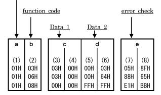
3) Communication answer format (MODBUS: Described by RTU because RTU is foundations) - The answer from a slave differs in message length along with a function code.
